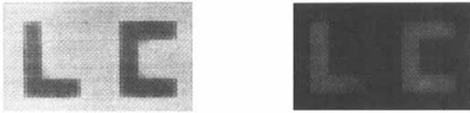
FIGURE 1 Optical images obtained by Monte Carlo simulations on 50 \times 30 \times 10 lattice. ( Left ): Twisted nematic display, ( Right ): In-Plane Switching display. The applied field strengths are \xi = 1 and \xi = -9 respectively.
